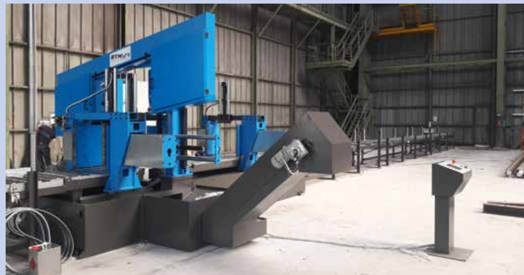
AP 7.6 TC 3 con rulliera in ingresso e uscita AP 7.6 TC 3 with infeed/outfeed roller track
