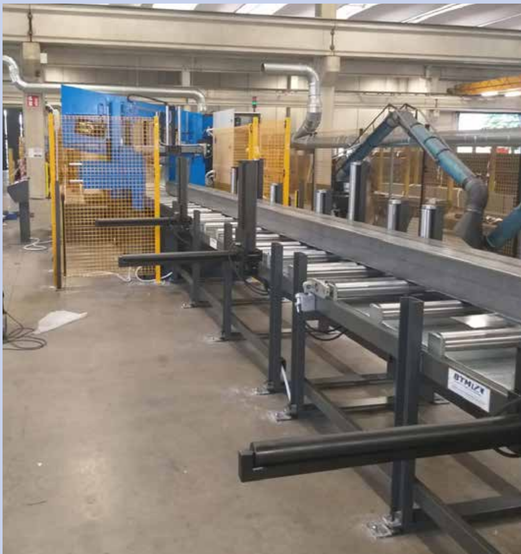
AP 7.6 TC 3 con rulliera in ingresso e uscita AP 7.6 TC 3 with infeed/outfeed roller track
