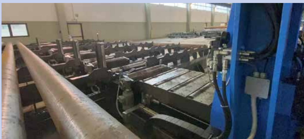
AT 740 TC completa di caricatore e rulliera uscita AT 740 TC with loading and outfeed roller track
