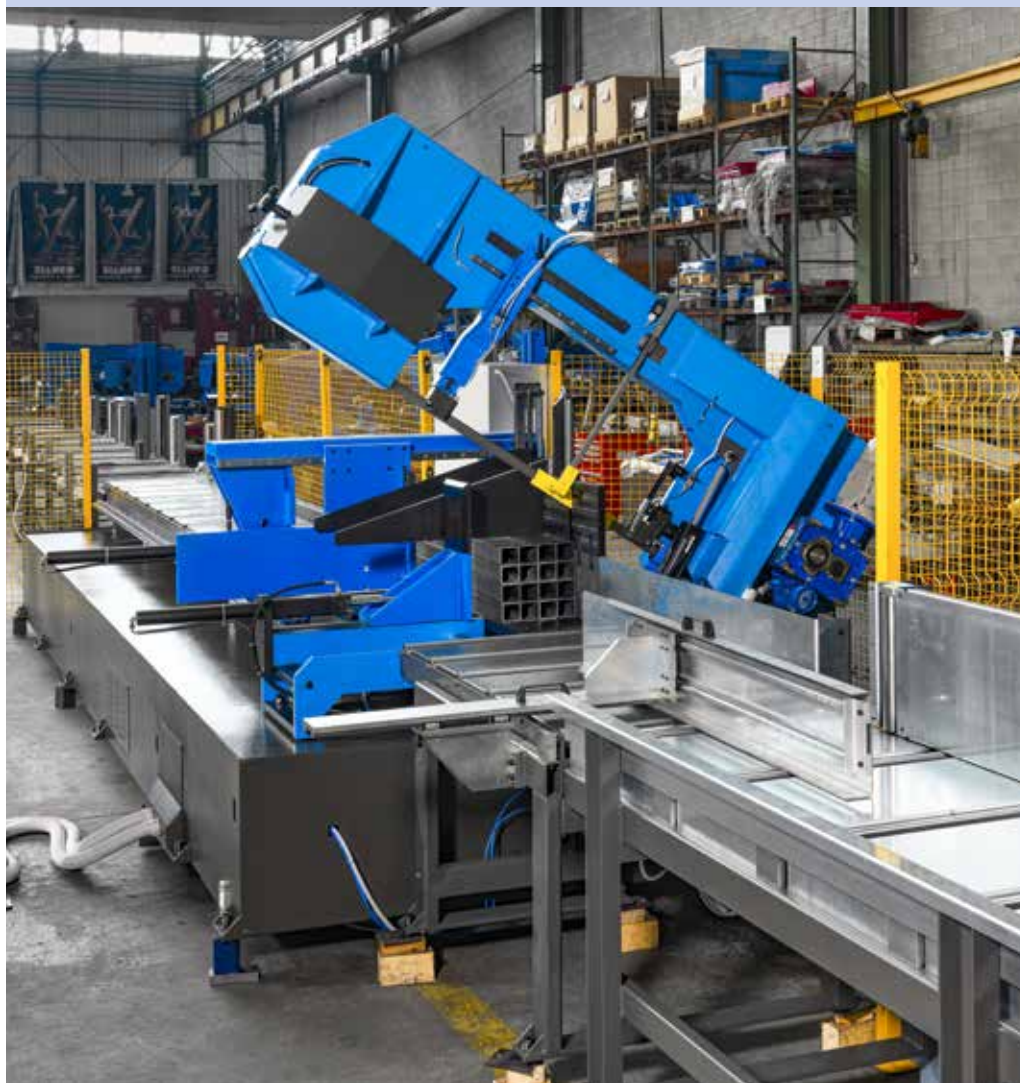
AP 7.5 A DS corsa carro 5500 mm con rulliere in ingresso e uscita AP 7.5 A DS carriage stroke 5500 mm with infeed and outfeed roller track
