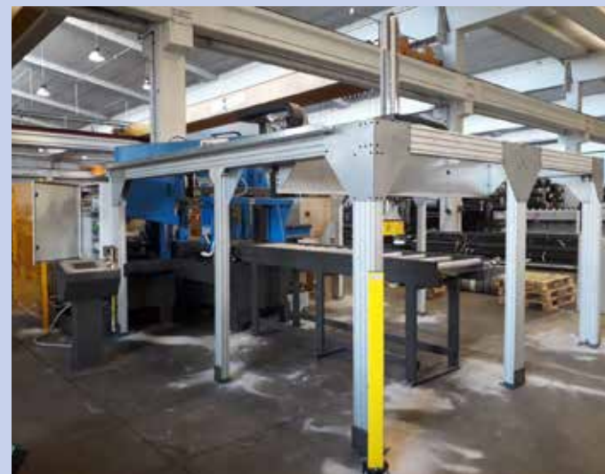
AP 7.5 TC 3 con rulliere e scaricatore a calamita AP 7.5 TC 3 with roller tracks and magnet unloading unit
