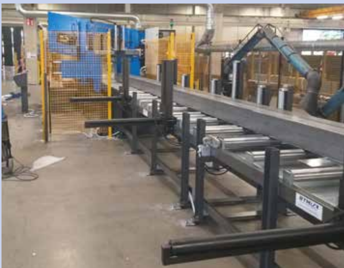
AP 7.6 TC 3 con rulliere in ingresso e uscita AP 7.6 TC 3 with infeed/outfeed roller track
