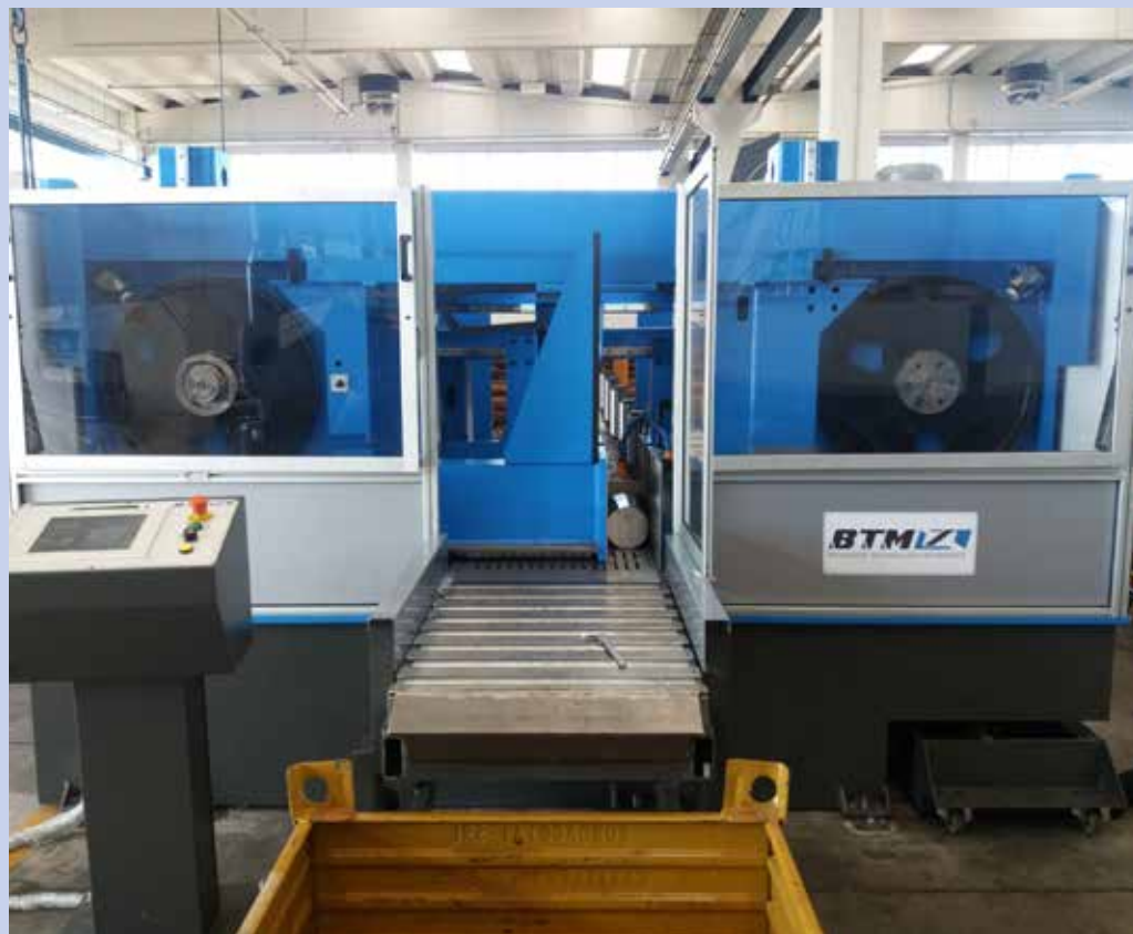
AT 640 TC con rulliera in ingresso e uscita AT 640 TC with in-outfeed roller track
