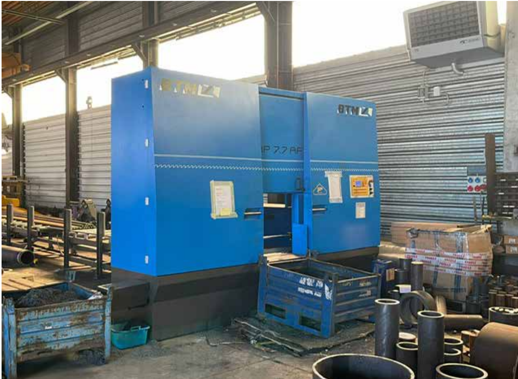
AP 7.7 AF con rulliera in ingresso AP 7.7 AF with infeed roller track
